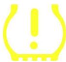
When cycling the ignition for off to run, the TPMS tell-tale should come on, and go off. This would indicate a system with no fault present.
